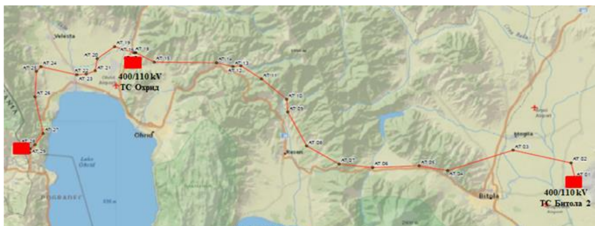
Figure 4. 400 kV interconnection TL SS Bitola 2 – Macedonian-Albanian border and SS 400/110 kV Ohrid route
