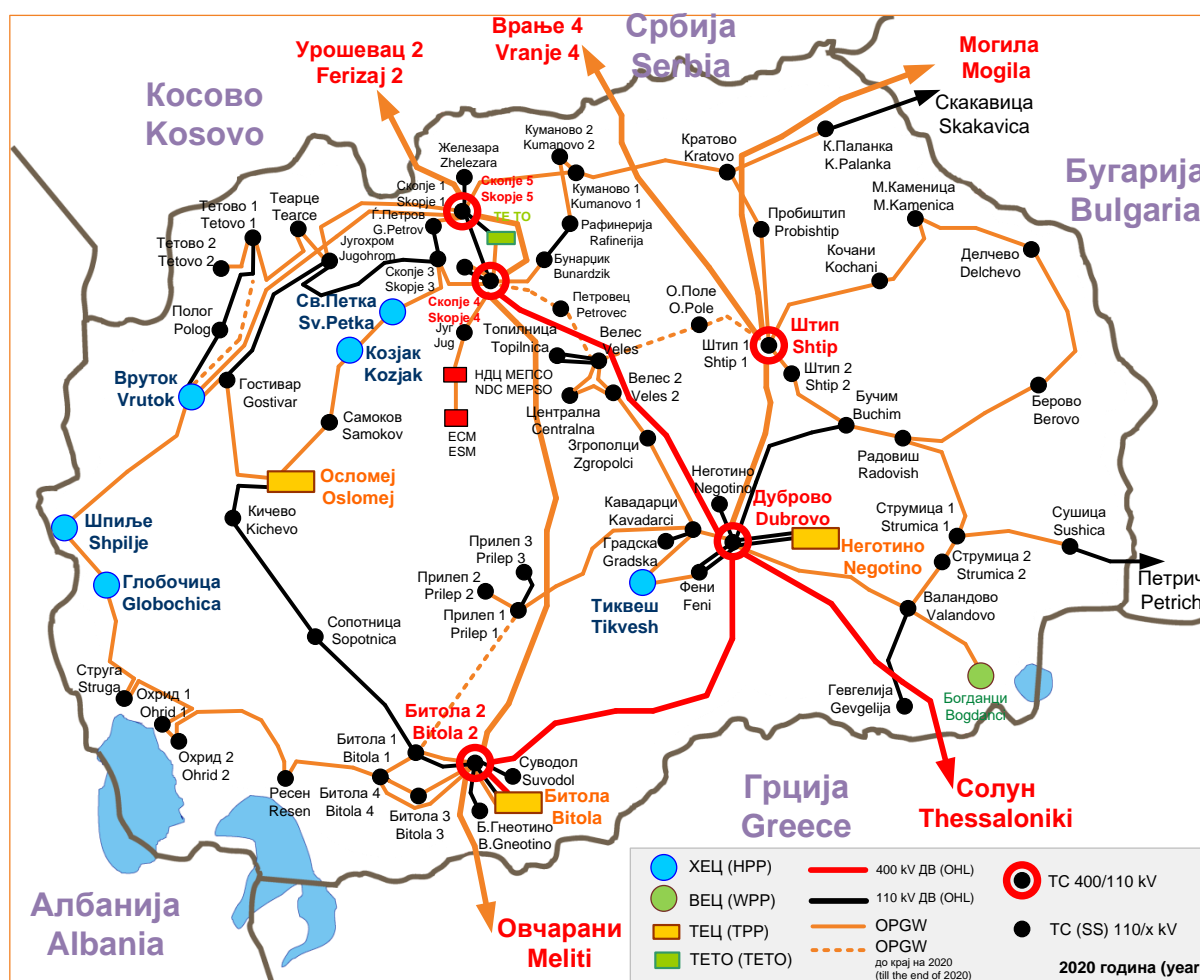
Figure 11. OPGW across the transmission lines of the transmission network
